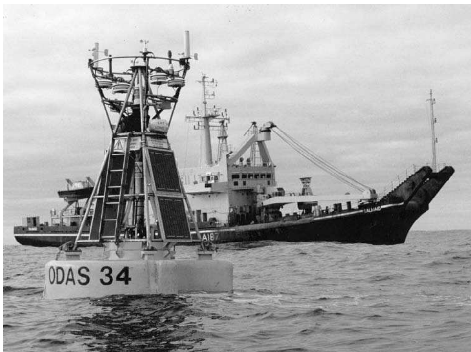
Figure 14.5 The UK Met Office operates nine deep-water buoys moored on the edge of the continental shelf in the northeastern Atlantic; the one illustrated is receiving a six-monthly service visit. This is similar to the TAO/TRITON buoys except that precipitation is not measured. Photograph reproduced by permission of the UK Met Office.
