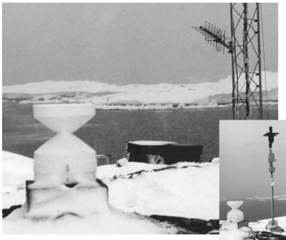
Figure 8.13 Being able to transmit observations from a remote site allows measurements to be received in near real time at a distant base. At this British Antarctic Survey site on the Antarctic Peninsula, readings are being telemetered via Meteosat. The electronic unit, known as a data collection platform, is housed in the box in the centre of the picture along with the battery power supply. The antenna is fixed to the mast on the right. An aerodynamic raingauge is near, left (see also Fig. 8.10e). This was part of an experimental cold-regions automatic weather station (inset) (Strangeways 1985).
