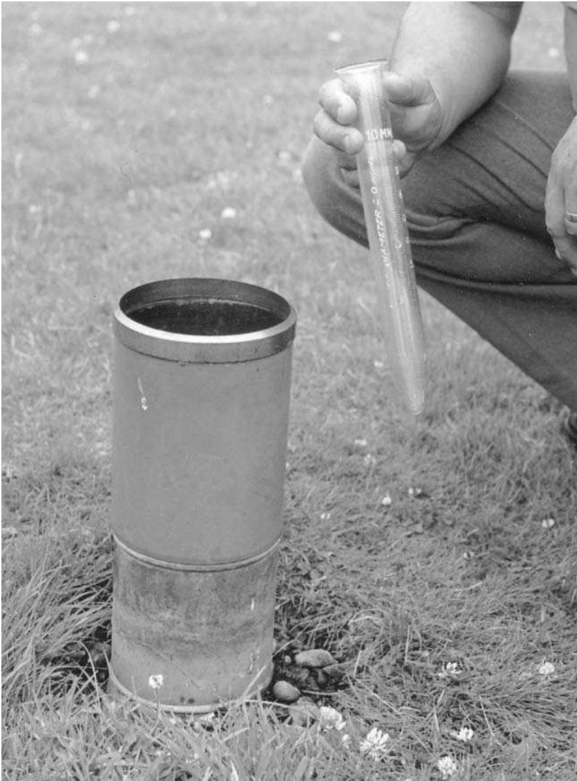
Figure 8.1 The UK Met Office standard manual raingauge is the 5-inch Mark 2. The collected water is stored in a bottle within the gauge and is measured daily with the graduated cylinder. The cylinder tapers at the bottom to help measure small amounts more accurately. The base of the gauge extends below the ground and splays out to give stability.
