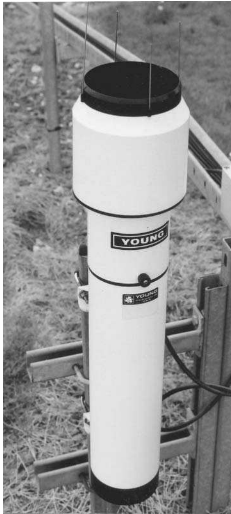
Figure 8.5 In this capacitance-based raingauge, the collected water is measured by storing it in a deep cylinder which contains two electrodes acting as the plates of a capacitor, the water between the plates performing the role of dielectric. By including the capacitor in a tuned circuit, the depth of water can be measured. As with other gauges that accumulate the water, it must be emptied periodically.
