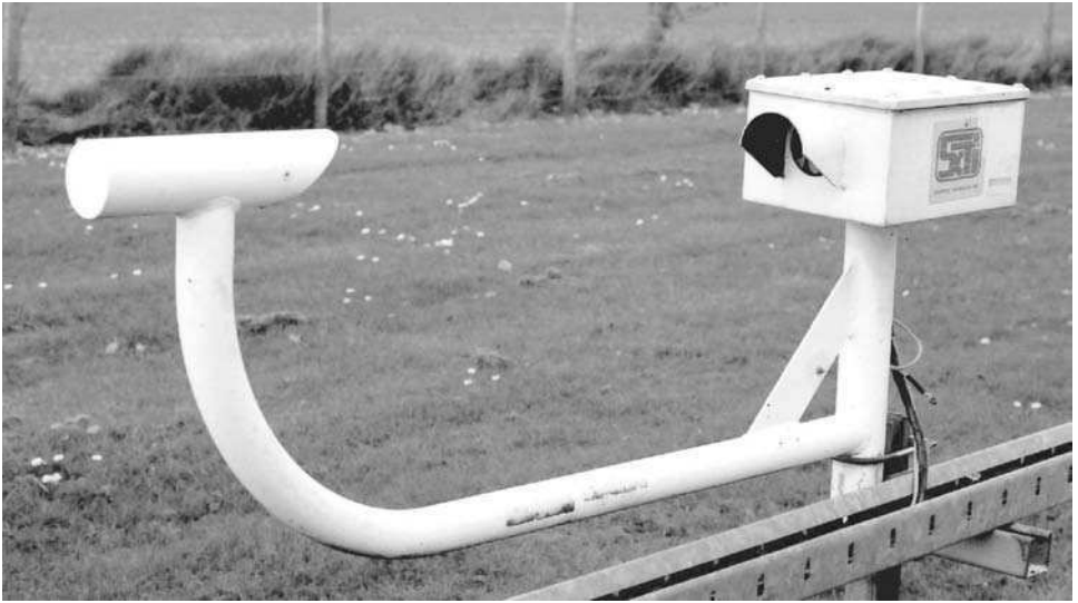
Figure 8.14 At the Rutherford Appleton field site at Chilbolton, this optical rain-gauge is used to detect rain intensity and drop size in radio propagation research. Optical gauges detect the precipitation passing through a beam of IR light passing between the source (right) and the detector (left) by analysing the scintillation produced by the falling drops. The nature of the fluctuations gives an indication of the intensity and type of precipitation, through complex algorithms.
