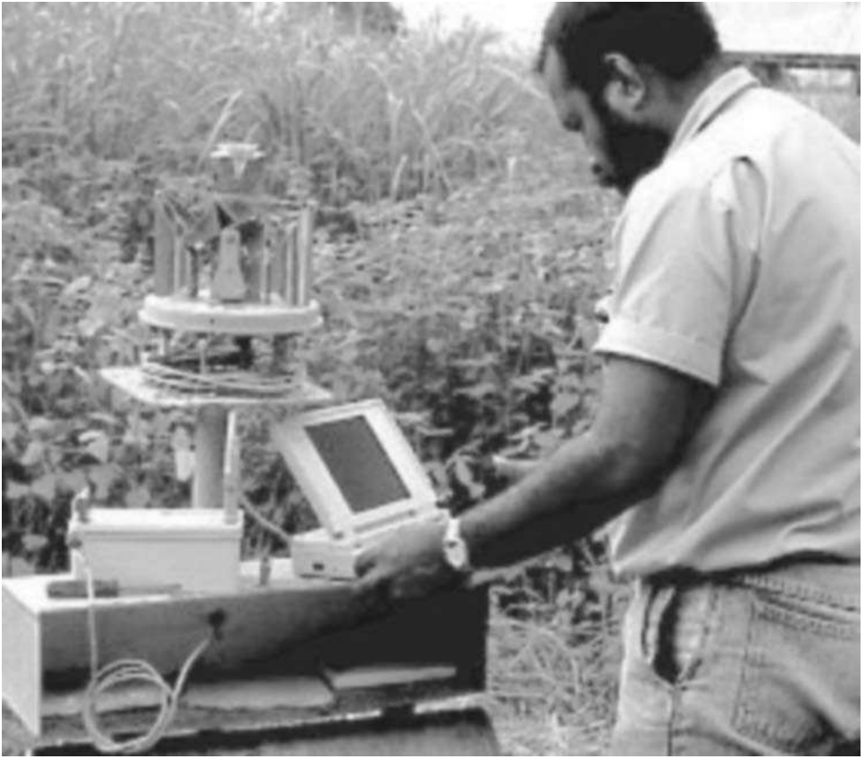
Figure 8.12 At this Papua New Guinea site, records from the tipping bucket raingauge (top) are being downloaded from a data logger (left) to a laptop.
