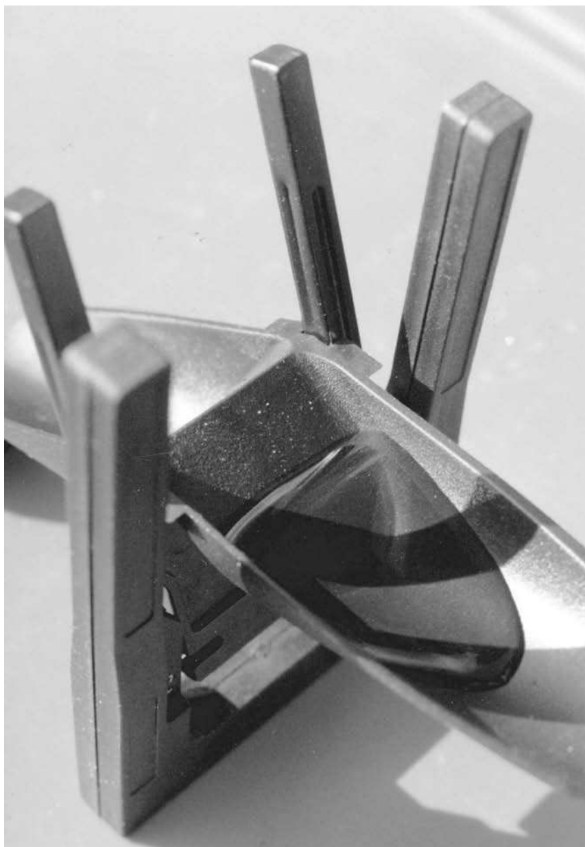
Figure 8.4 Today, the most usual way to measure the water collected by a raingauge is by tipping bucket. If the collector is 500 \text{ cm}^2 in area, 0.2 \text{ mm} of rain produces 10 \text{ ml} of water. As the bucket tips, a magnet in the moving arm momentarily closes a reed switch in the fixed outer arm, producing pulses that can be recorded, most usually by a data logger.
